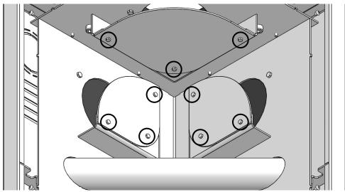
Fig. 10 Chimney cleaning instructions - unscrewing
