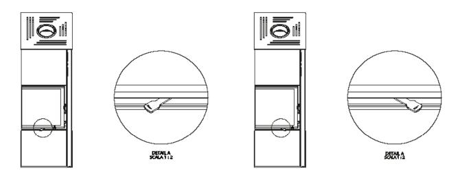
Fig. 8 Throttle operation - moved to the right - air supply closed, moved to the left - air supply open.
