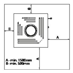
Fig. 7 Safe area for flammable materials
