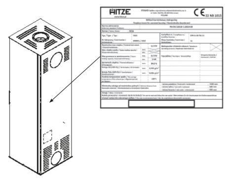
Fig. 12 The model of the nameplate and its location
