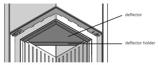
Fig. 9 Instructions for cleaning the chimney - removing the deflector
