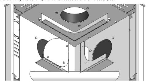
Fig. 11 Instructions for cleaning the chimney - flue pipes
