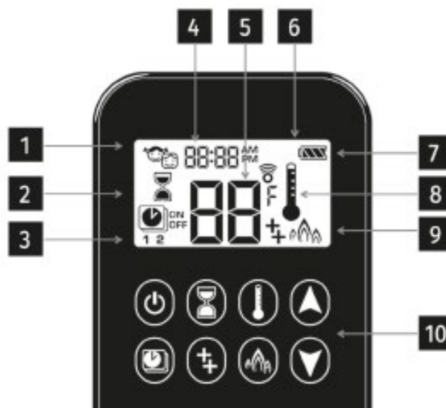
Fig. 10. SYMAX (MAXITROL) remote control: 1 - Child Proof, 2 - Timer mode, 3 - Program mode, 4 - Hour and minute field, 5 - Ambient temperature, 6 - Display, 7 - Battery indicator, 8 - Thermostat mode , 9 - ECO Mode, 10 - Buttons
