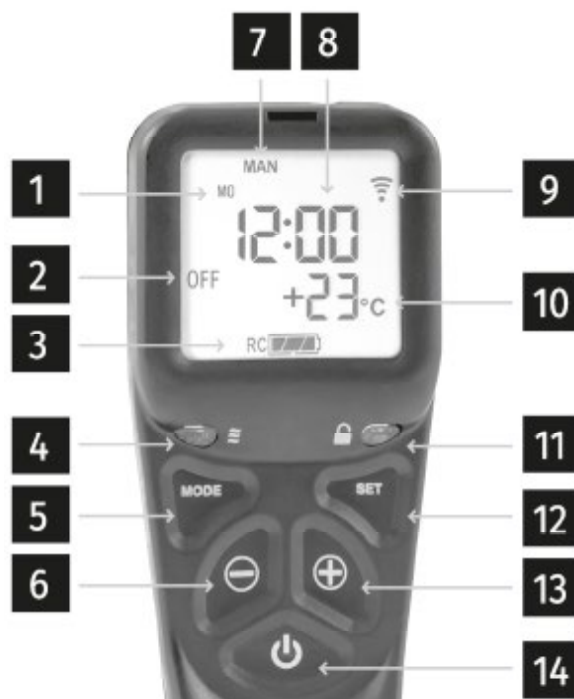
Fig. 11. Remote control type FB 868D (TESC) 1 - Day of the week, 2 - Heater status, 3 - Battery indicator, 4 - Light sensor, 5 - Mode selection, 6 - Decreases the flame button, 7 - Current mode, 8 - Hours and minutes field, 9 - Connection with the heater indicator, 10 - Ambient temperature, 11 - Remote control lock indicator, 12 - Entering settings, 13 - Increase the flame button, 14 - Turn on / off
